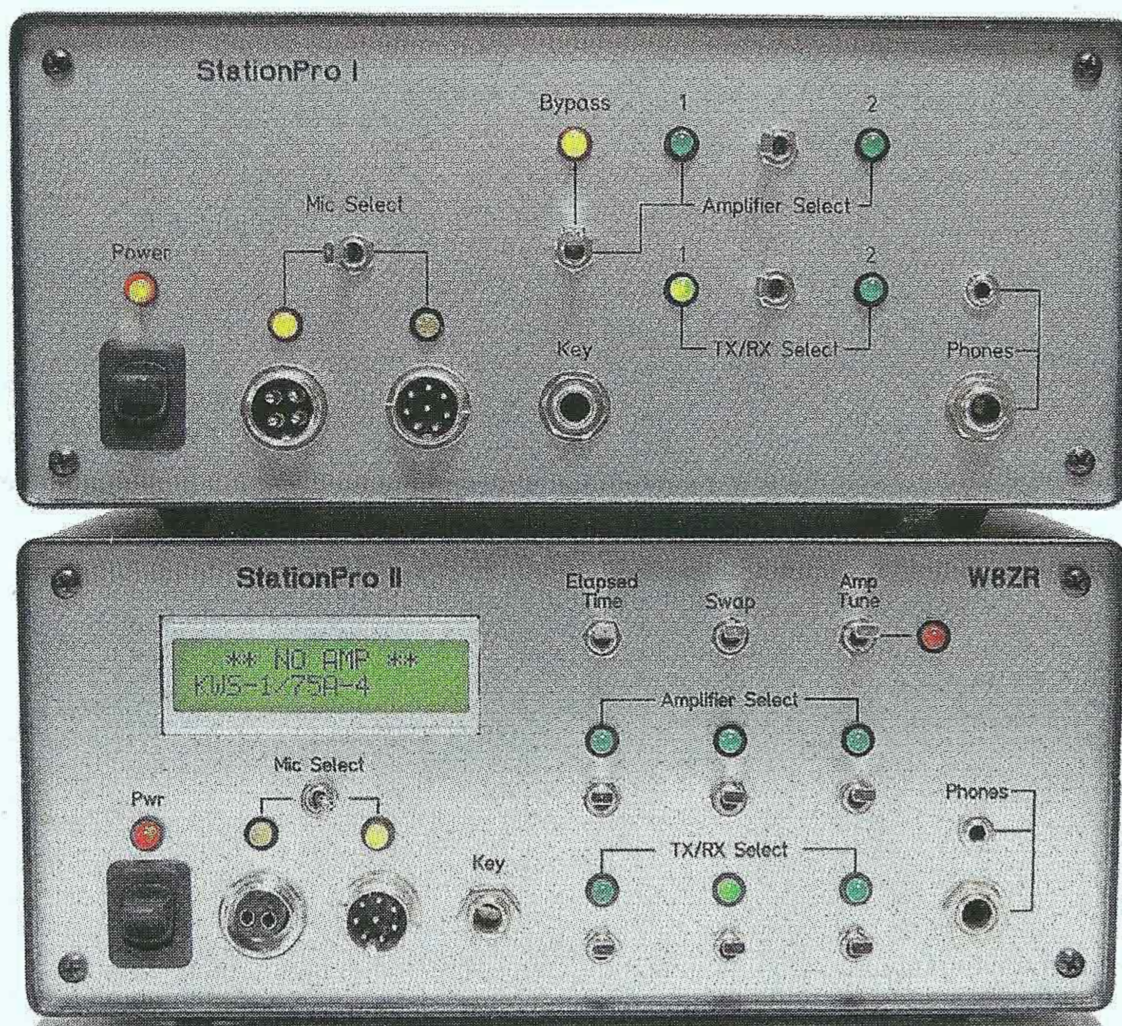
Figure 1 — The StationPro comes in two versions. The SP-I (top) handles the switching for two transceivers and linear amplifiers, while the deluxe SP-II version accommodates up to three transceivers and amplifiers.
